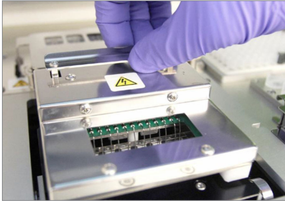
FIGURE 5.29: Releasing the fixture after a completed run
